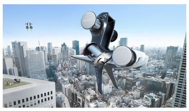
For the first time, the unique characteristics of CycloRotors were used to design a mission optimized unmanned cargo eVTOL, compact in size, stable in windy weather with precision landing capability into confined areas of 5 m in diameter, and capable of transporting 45 kg payload over a distance of 40 km.
